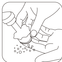
3. Rinse the filter and air inlet mesh with tap water to remove dust and hair residues.
